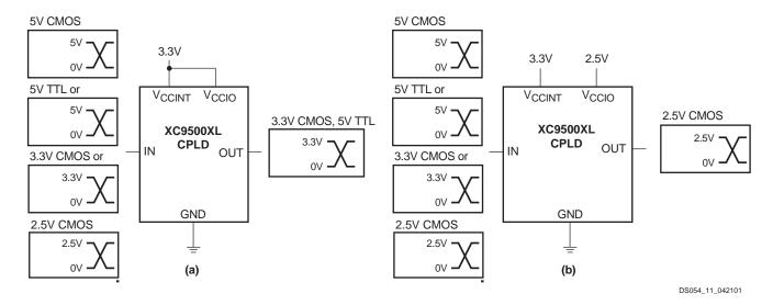
Figure 11: XC9500XL Devices in (a) 3.3V only and (b) Mixed 5V/3.3V/2.5V Systems
