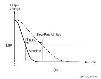
Figure 12: Output Slew-Rate Control For (a) Rising and (b) Falling Outputs
