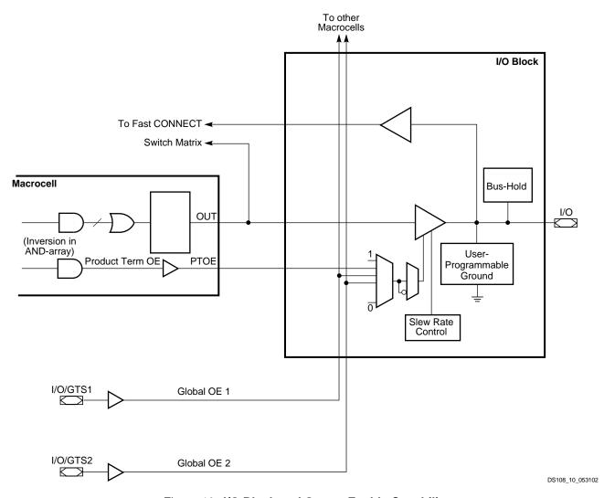
Figure 10: I/O Block and Output Enable Capability
