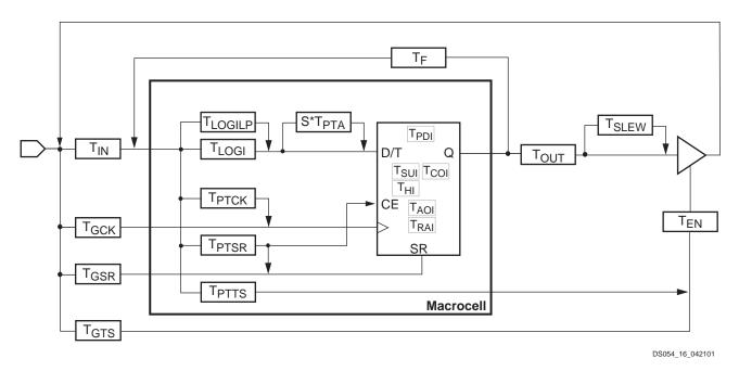
Figure 16: Detailed Timing Model
