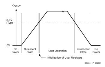
Figure 17: Device Behavior During Power-up
