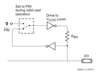
Figure 13: Bus-Hold Logic
