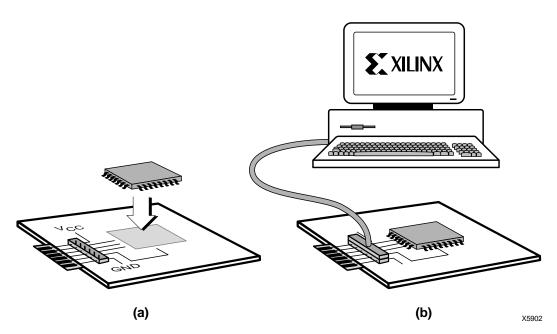
Figure 14: System Programming Operation (a) Solder Device to PCB and (b) Program Using Download Cable
