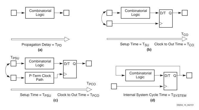
Figure 15: Basic Timing Model
