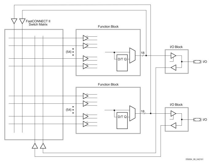
Figure 9: FastCONNECT II Switch Matrix
