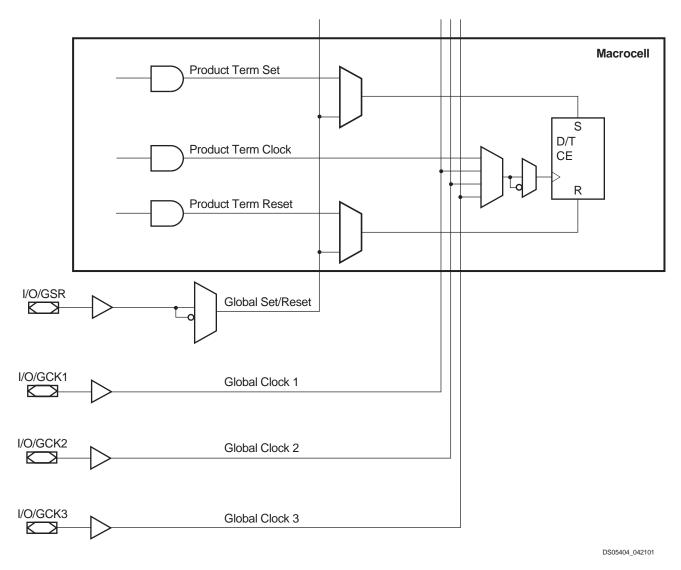
Figure 4: Macrocell Clock and Set/Reset Capability
